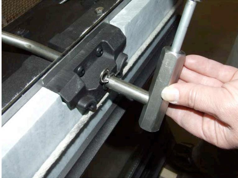
7. Locate the push pin on the shaft on the front side of the stove. Tap it through with a hammer and punch as far as you can. Pull it out the opposite side with locking pliers.
