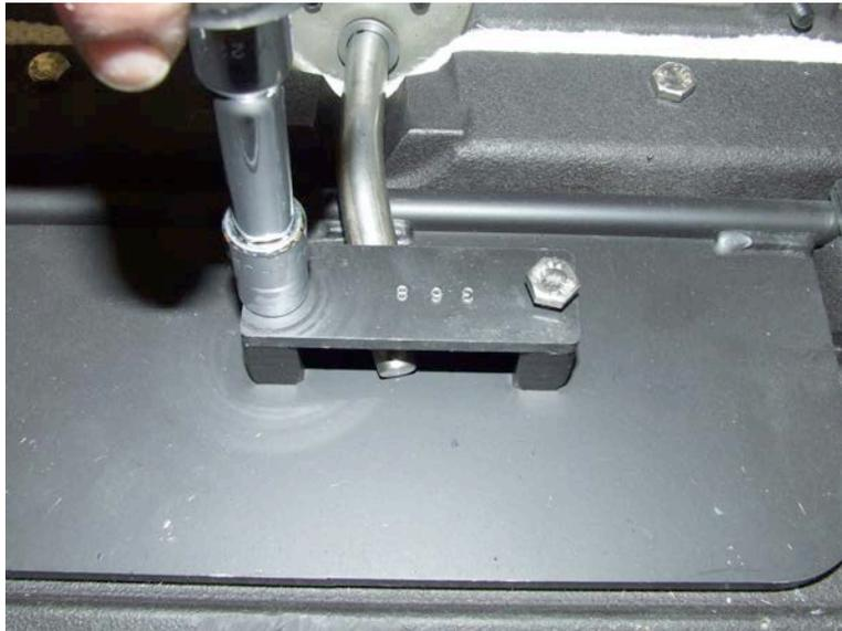
9. Pull the bypass shaft out of the stove by pulling the shaft inward toward the back of the stove.
