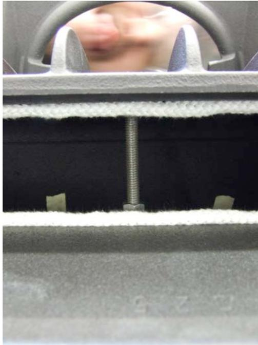
39. 12. Install the by-pass activation rod through the escutcheon and body box with a spacer on each side. Drive a 1/8" x 3/4" roll pin through each hole in the rod to secure it in place. Secure the bypass handle to the rod. Make sure it is in the proper position to indicate whether the bypass is open or closed.
