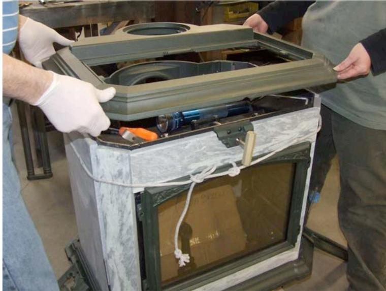
40. Carefully place the top cast onto the stove body. Be sure the draw rod bosses clear the exterior stones.
