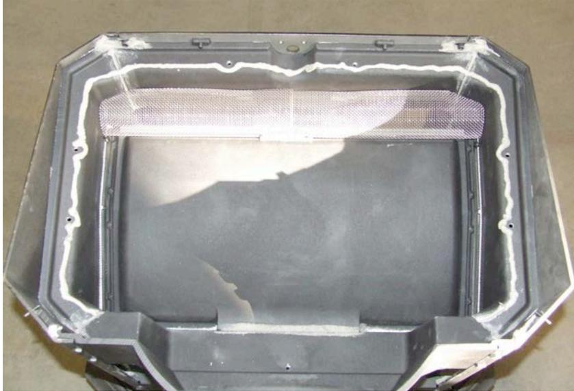
29. Lower a catalyst base/by-pass plate (P-325) into place on the stove cement as shown below and secure with (4) 1/4-20 x 3/4 HHCS in the front 4 bolt holes, loosely for now.
