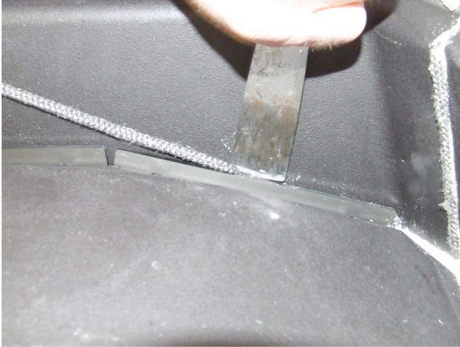
20. Cement the space inside the firebox where the secondary air chamber penetrates the rear wall. Wipe smooth with finger.
