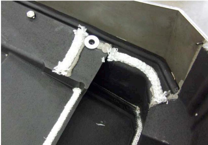
33. Lay the catalyst top upside down on your work bench. Lay a line of gasket glue in the catalyst gasket track and put .250" gasket in the track with an extra 1" of
