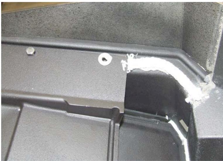
31. Run a line of gasket glue in the cat gasket channel of the catalyst base. Only put the glue on the horizontal channel, not the vertical yet. Run .250" gasket in the horizontal part of the channel only.
