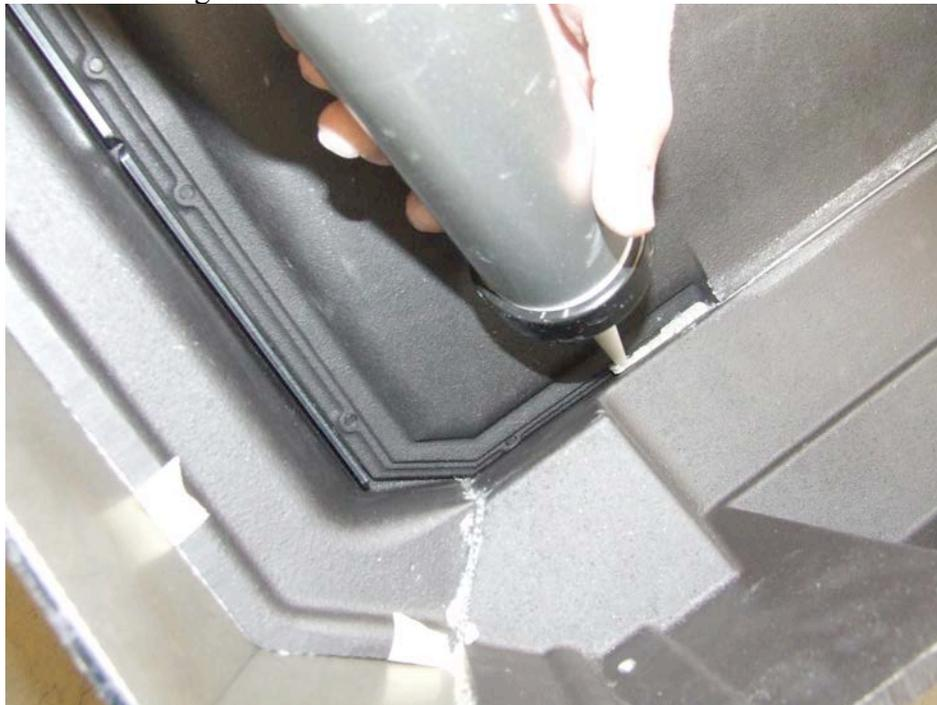
19. Place .187" gasket ( or .250" if gap is wider) along the sides of the secondary air chamber from the rear to the front as shown here.
