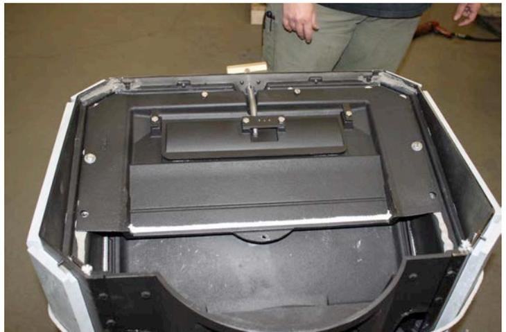
30. Place .312" gasket on top of the stove cement that the catalyst top will sit on.
