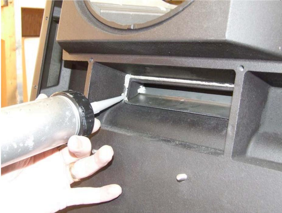
22. Place .187" gasket in this cement then apply a generous amount of cement over the gasket and smooth with your finger.
