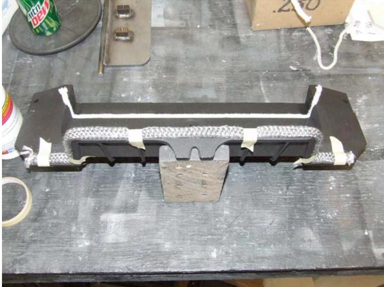
35. Lower the catalyst top (P-326) into place and secure the wings with (2) 1/4-20 x 1" HHCS and a 1/4" washer. Make sure the tab at the rear of the catalyst top is inside the lip of the rear wall as shown.
