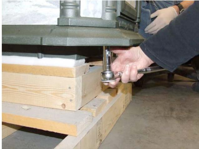
4. Locate the four Allen nuts that fasten the cast front to the stove. There are two on each side of the frame.
