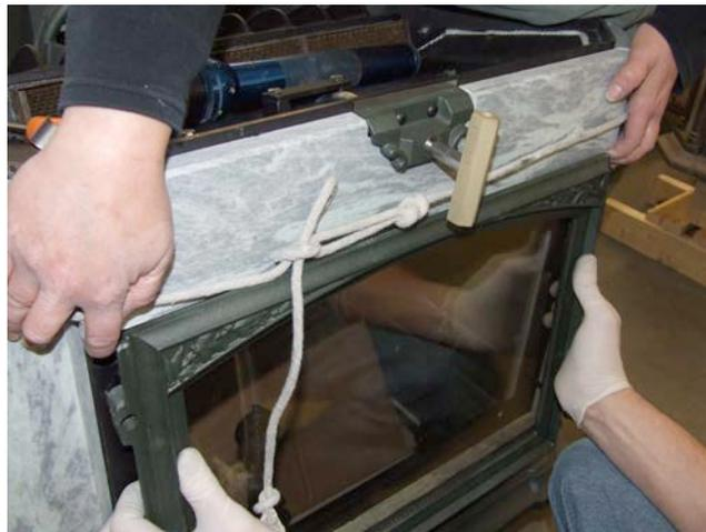
6. **Note:** The assembly consists of a cast iron frame and two panes of glass. On top of the assembly sits the over the front stone that will also come loose when the front assembly is removed. If the stone is dropped it may be damaged. One person should hold the stone upward while the other removes the front assembly.
