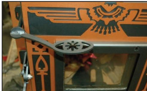
*The bypass lever interlocks with the door when the combustor is engaged (bypass closed). This safety feature makes it impossible to open the loading door without opening the bypass.*
