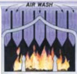
A curtain of preheated primary combustion air falls down over the window
