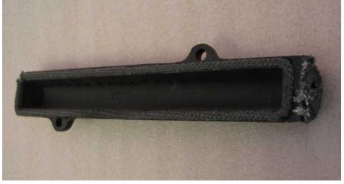
14. Attach the air tube to the baffle using the two 1" long bolts from inside the firebox and fastening with a washer and nut on the top side of the baffle.(Your replacement baffle has this hardware pre-attached. If you attach the secondary air tube, you will have 2 flat washers left over.) If the slots in the baffle are not covered completely by the washer fill the hole with some furnace cement.
