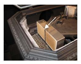
17.Replace the 1/4" gasket on the bottom side of the combustor hood using gasket glue.
