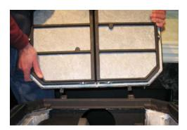
3. If your stove has one, remove the stainless steel deflector from the cast iron hood, using a 7/16" wrench or socket. Remove the cast iron combustor hood by removing the two bolts using a 1/2" wrench or socket on the top side of the baffle plate and another 1/2" wrench on the nuts on the bottom side of the baffle plate. Remove the combustor and hood.
