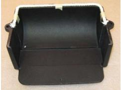
18.Install the combustor hood and place the two bolts down through the hood and into the baffle for alignment. You do not need to tighten the bolts with nuts. The nuts are only needed for shipping the stove. Replace the stainless steel deflector, if you have one.
