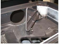
6. Remove the secondary air tube from the firebox side of the baffle by holding the bolt in the firebox with a wrench and turning the nut on the top side of the baffle with a socket and lower the tube off the baffle (Alternately, you can do this step after you have completely removed the old baffle).
