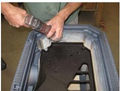
12.Replace the two eyebolts making sure they are properly seated over the tab on the vertical supports. Fasten them using the nuts and a 9/16" socket and 6" extension.
