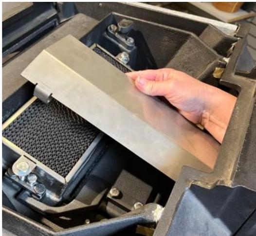
6. Remove retaining bolts (if installed) with a 1/2" socket or wrench from tabs on both sides of the catalytic combustor.
