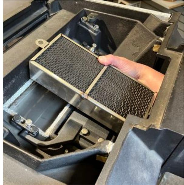
8. Inspect the under combustor gasket and replace if needed- a good seal under the catalytic combustor is critical to proper performance and efficiency. See our website ([www.woodstove.com](http://www.woodstove.com)) or call us at 800-866-4344 to order a new under combustor gasket kit, which includes a proper length of gasket and the gasket glue to install it.
