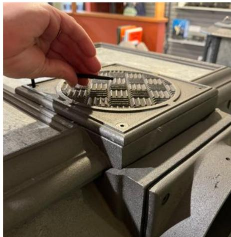
3. Close the bypass cover by lifting up the bypass lever (the shaft on the back of the stove with the black knob on the end).
