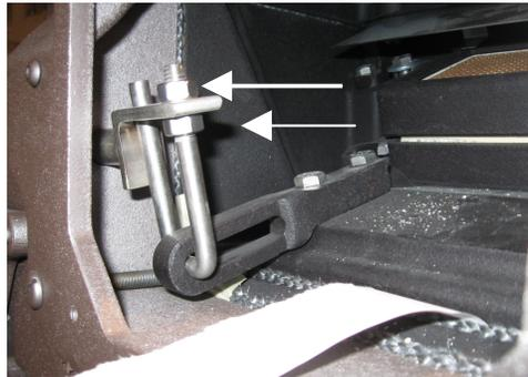
When properly adjusted, you should have to apply some pressure to the bypass lever to close the cover completely.
