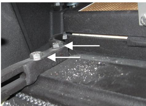
3. Install the new lift guide with the supplied bolts. Apply anti seize compound to the threads of the bolts.
