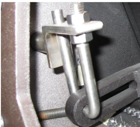
5. Test the seal between the bypass cover and the gasket using a slip of paper. Close the bypass cover on the paper. There should be enough resistance on the paper to slightly curl it when it is pulled out. To increase pressure on the bypass door, loosen the top nut on the U-bolt, and then turn the bottom nut counter clockwise. To decrease pressure on the bypass door turn the bottom nut clockwise, and do the same to the top nut. Make small adjustments until the proper seal is reached.
