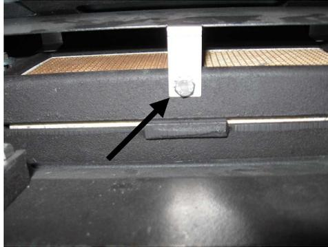
4. Remove the catalytic combustor from the stove. If you have not already done so remove the transport bolts with a 1/2" wrench. The bolts do not need to be returned to the stove. Turn the combustor 90 degrees to remove it. Remove the gasket from around the combustor opening in the combustor pan. Use a putty knife and wire brush to remove any residual gasket or glue. Vacuum up any loose debris.
