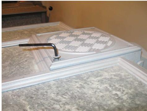
3. Remove the heat shield from the catalytic combustor frame with the 7/16" socket or wrench. Use caution as the edges are sharp.
