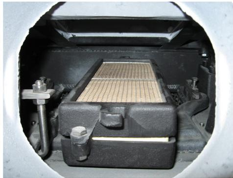
5. Dry fit the replacement gasket. Start in a corner and lay the gasket into the gasket channel until you are back to the starting point. Cut off excess gasket with sharp scissors if necessary. Set gasket aside.
