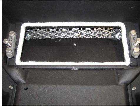
8. Return the catalytic combustor to the stove. The open side of the hooks for the transport bolts should face the back of the stove. Carefully install the heat shield onto the combustor frame.
