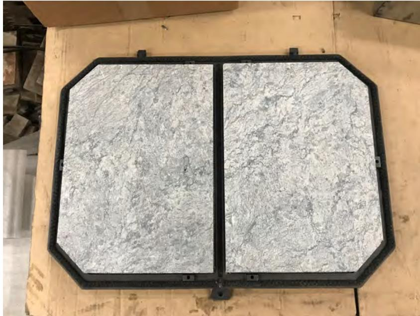
10. If the stone rests on the cast iron not the gasket, use a sander or flat file to remove stock from the edge of the two areas indicated in the following photo. Only remove enough to ensure a good fit (Maximum of 1/16")
