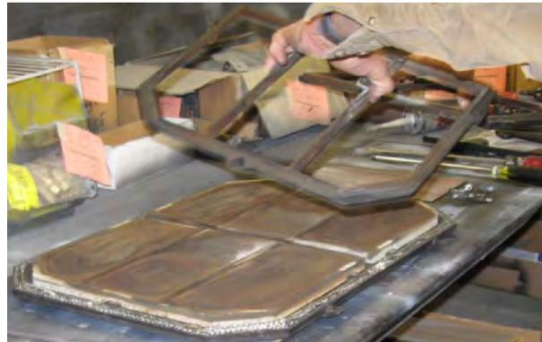
6. Remove the stone(s) to be replaced. Push the stone(s) up and out of the frame from below.
