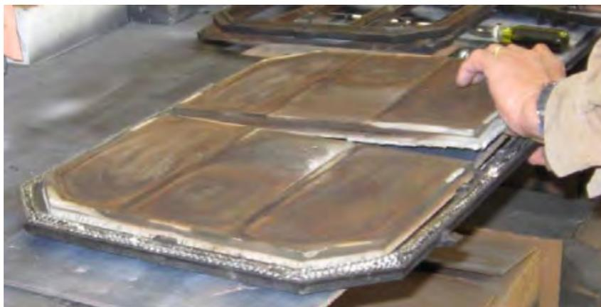
7. We recommend replacing the stone gasket at this time. Remove the gasket that rests under the stone(s). Use a putty knife or flat blade screwdriver to clean the residue from the frame as much as possible.
