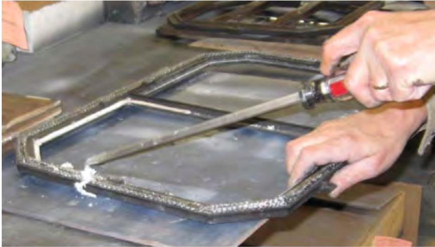
8. Apply a small bead of gasket glue to the frame and install the gasket. Use a putty knife or flat-blade screwdriver to help seat the gasket into the gasket channel. Do not allow the glue to dry before the gasket is in place or it will become hard and lumpy.
