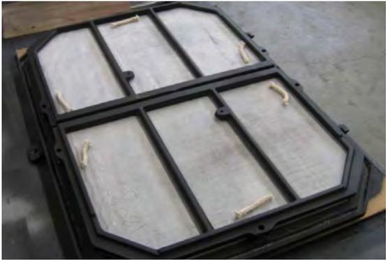
12. Tighten the screws evenly. Give each screw a few turns and repeat around the frame. Tighten the screws snugly, but do not over-tighten as this may lead to broken stone. With the screws completely tight you should be able to squeeze the retainer toward the lid and have no visible motion.
