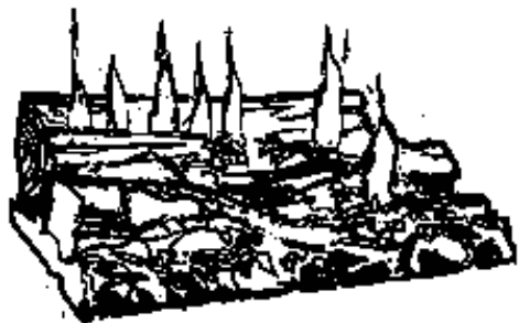
Illustration 21.1 When the burner is clean and the Fireplace is operating properly, the flame pattern will look approximately like the drawing above.
