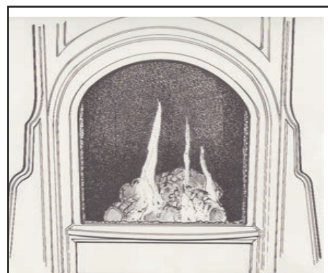
When the Mini is operating properly, the flame pattern will look approximately like the drawing above.
