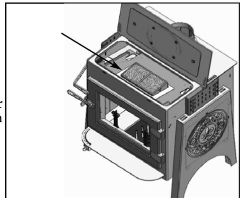
*The Catalytic Combustor is easily accessible. Just lift the lid, remove the radiator using the two finger holes, and the catalyst is visible. The catalyst can be removed by lifting the catalyst housing.*
