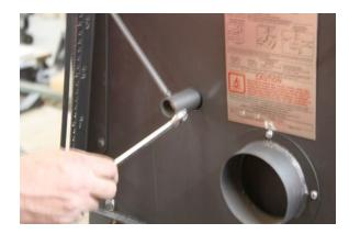
3. The rear panel of the stove is fastened in 7 places. Use a 7/16" wrench or socket to remove all the nuts, bolts, and washers.
