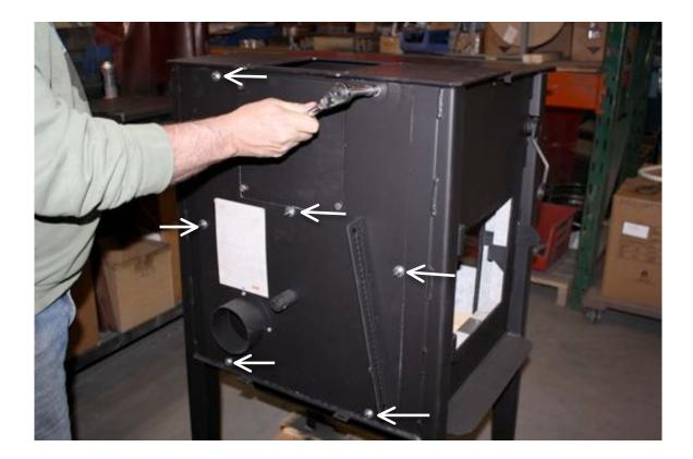
4. Remove the back panel of the stove to expose the two air jets.
