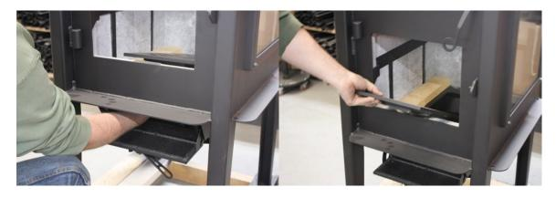
7. With the ash grate out, remove the 3 pieces of firebrick from the rear wall of the stove.
