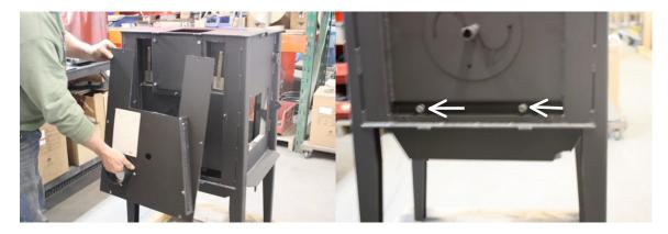
5. Use a 3/4" socket to remove the 2 air jet bolts. Set aside.
