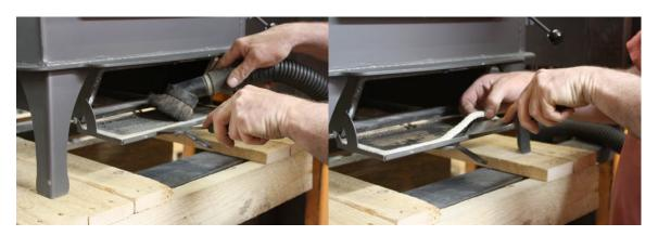
Squeeze out a roughly 1/8" bead of glue all around the gasket channel on the door. Starting in the middle of the back, place the gasket into the channel and glue, pushing back on itself slightly to give it some "fluff".
