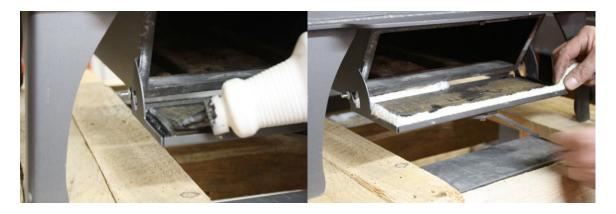
When you get back to the starting point, trim the gasket so that the ends butt together. Close the door firmly (without latching) 2 or 3 times. Place a strip of paper (or a dollar bill) on the gasket and close, and latch, the door. You should feel some tension when you try to pull out the paper, and it should curl slightly. Repeat this in several places around the door.
