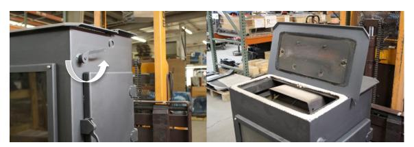
Start by removing the old gasket, then, using a putty knife (or wire brush) and shop vac, clean out the gasket channel of residue from old gasket and dried glue.
