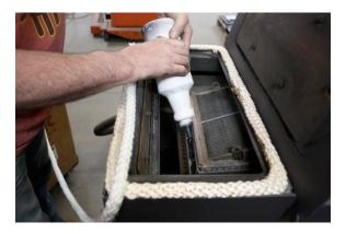
Starting in the front corner, opposite the bypass handle, lay the gasket into the channel and glue, stretching slightly along the front channel ONLY. The remaining three sides should be installed without stretching, particularly in the corners. When you get back to the starting point, trim the gasket so the ends just butt together.
