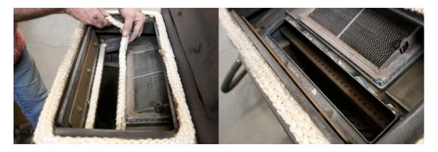
Squeeze out a bead of glue (about 1/8") all around the gasket channel.
