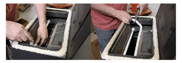
Place a strip of paper (or a dollar bill) on the gasket and close the bypass door. You should feel some resistance when you try to pull out the paper and it will curl slightly.
