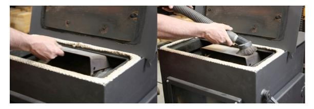
Remove the old gasket from under the combustor, then use the putty knife (or wire brush) and shop vac to remove any old gasket and glue residue.
