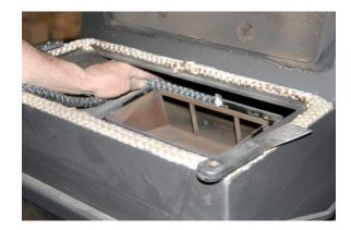
Place the combustor back into the stove making sure the welded side is up and the combustor angles toward the front of the stove. Replace the shield, making sure the 2 round holes in the shield are towards the front of the stove and the shield "legs" are in the notches in the flat flange of the combustor.
