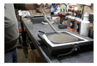
Use a putty knife (or wire brush) and a shop vac to clean out any residue of old gasket and dried glue.
