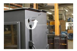
Open the loading door. Get a firm grip on the door (it's HEAVY) then remove the hinge pins to release the door (you may need to wiggle the hinge pins to pull them out). Place the door flat on a bench so you can work on it.
