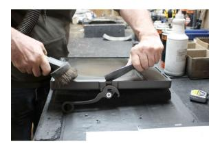
Squeeze a bead of glue (about 1/8") all around the gasket channel. Starting at the center of the bottom, lay out the gasket all around the door. Start inserting the gasket into the channel (be careful not to stretch it, particularly in the corners) and tuck in the edges with a putty knife.
