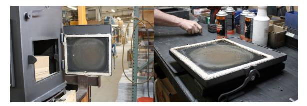
Use a putty knife to pry out one end of the old gasket then pull on it to remove completely.
