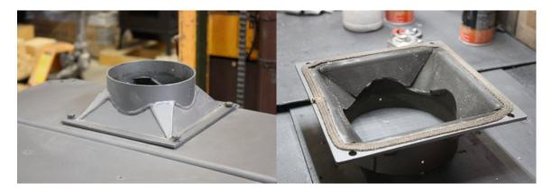
Pull off the old gasket and, using a putty knife (or wire brush) and shop vac, clean the surface of any residue.
