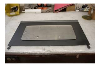
2. Using a 7/16" wrench or socket, remove the 6 hex nuts from the bolts. Lift the heat shield straight up to remove. Then remove the 6 heat shield spacers and set the shield, the nuts, and spacers aside.
