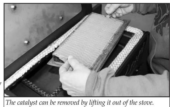
5. Return the combustor to the stove. Be sure that it is seated properly. Place the heat deflector over the combustor.
