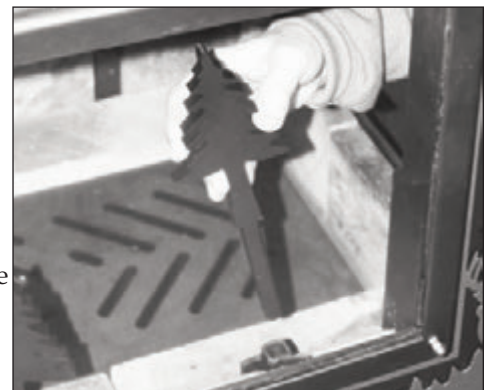
Insert the andirons back into the stove after cleaning the glass. The andirons help keep wood away from the glass and the air wash system unobstructed.
