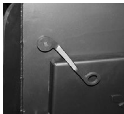
The bypass lever interlocks with the door when the combustor is engaged (bypass closed). This safety feature makes it impossible to open the loading door without opening the bypass.
