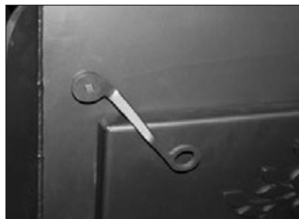
The bypass lever interlocks with the door when the combustor is engaged (bypass closed). This safety feature makes it impossible to open the loading door without opening the bypass.
