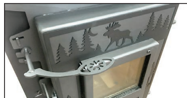
The bypass lever interlocks with the door when the combustor is engaged (bypass closed). This safety feature makes it impossible to open the loading door without opening the bypass.
