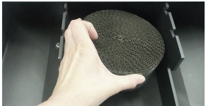
Lift the catalytic combustor out and clean both side (see instructions to the left).
