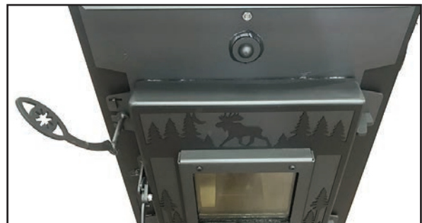
Bypass lever should be up when starting or reloading the Survival Hybrid, allowing the smoke to heat up to 500° internally, or 200°-250° on the surface.
