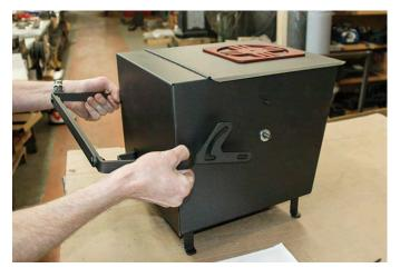
5. Apply the nylon insert lock nuts and tighten. Do not over-tighten. The handle should move freely back and forth, and up and down.
