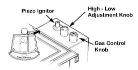
*Piezo:* This is an igniter that lights the pilot by creating a spark. It is the same type of lighter that's found on home barbecue grills. A match or flame is not required to light the pilot.
