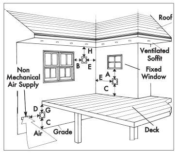
Horizontal termination caps must be positioned 12-18 inches above grade, and 12-18 inches away from windows, decks, soffits, and non-mechanical air supplies.
