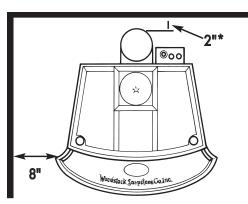
Minimum Clearances: Parallel Installation \* 2" clearance can only be achieved with a straight-up vertical vent configuration.
