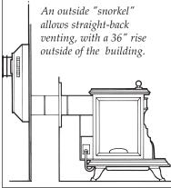
and minimum inner flue diameter of 6".
