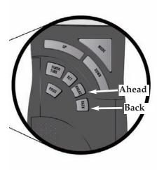
1. On your Transmitter, press the **Ahead** and **Back** buttons simultaneously to display the swing setting. (It will flash off and on).
