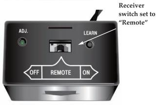
5. Check to see if the transmitter is out of range from the receiver (15 – 20') Move the transmitter closer to the receiver and try again. If the transmitter works near the stove, but not further away, it could simply be a weak battery problem.
