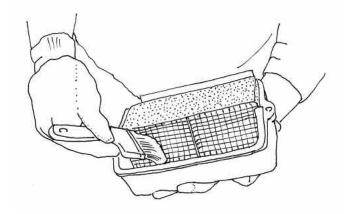
Fly ash should be removed from the catalytic combustor cells periodically with a vacuum cleaner or a soft brush.
