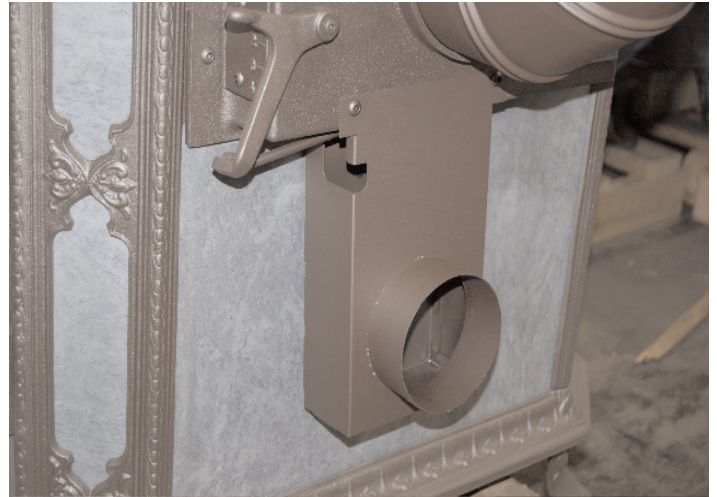
The Outside Air Adapter attaches to rear of stove over the air damper inlet. The four inch round outlet allows you to connect ducting from the stove to the outdoors.
