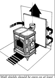
Wall shields should be open on at least three sides to allow for air flow.
