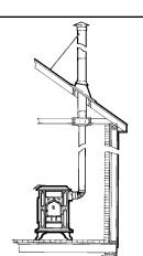
A chimney that stays inside the house as long as possible will perform better than one that runs through the wall and along the outside of
