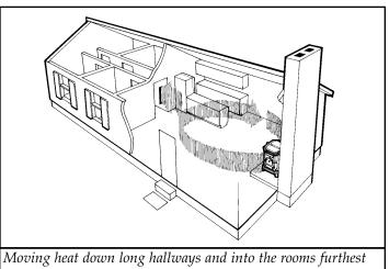
Moving heat down long hallways and into the rooms furthest from the stove is more difficult. Sometimes cold air returns or doorway fans can help.
