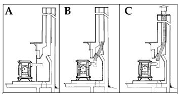
Illustration A above depicts the worst possible fireplace installation - leading to creosote and backpuffing. B is a halfway point - a flexible pipe runs just up to the point where the chimney's tile liner starts. C is the best fireplace installation - one full liner from top to bottom. These liners come in kits complete with cap, top plate, tee and flexible stainless steel liner.
