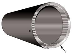
The MALE end is the inner crimped end, and points down, or toward the stove
