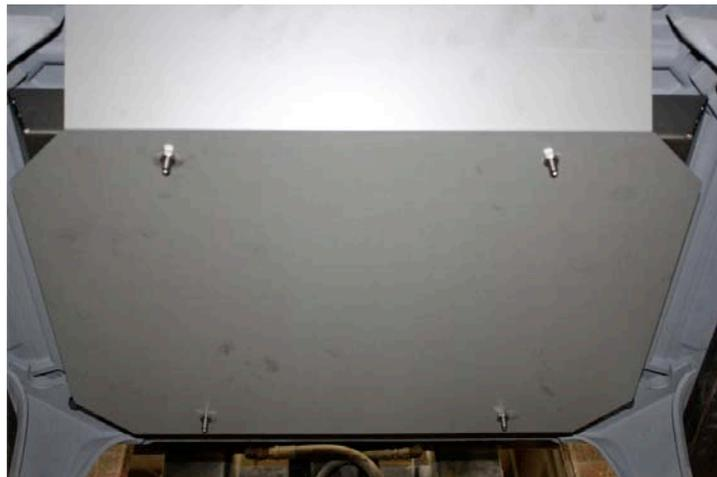
6. Place the #3 shield on the four threaded studs, paying attention to it's orientation (UP and arrow). Turn a 1/4-20 nut on to each stud just enough to hold the shield in place.
