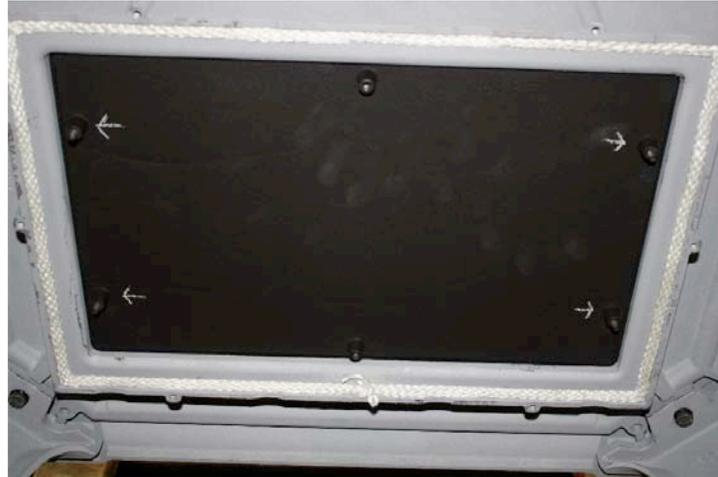
3. Insert the 4  $\frac{1}{4}$ -20 x 1  $\frac{3}{4}$ " long threaded studs into the front and rear holes on the bottom of the stove's base. Snug them up with a  $\frac{1}{8}$ " allen wrench.
