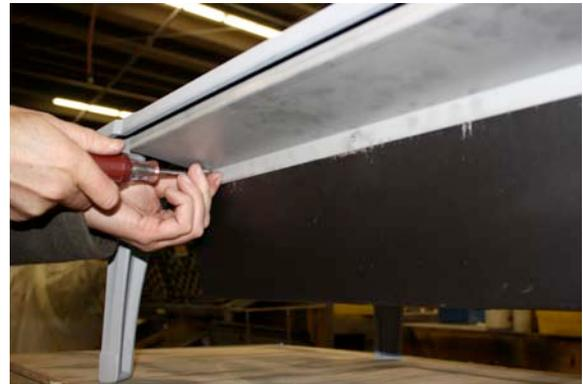
5. Repeat step #4 for the rear shield extension. After installing the rear shield extension go back and fully tighten all of the sheet metal screws to secure the ash pan shield and front and rear extensions to the ash pan holder.
