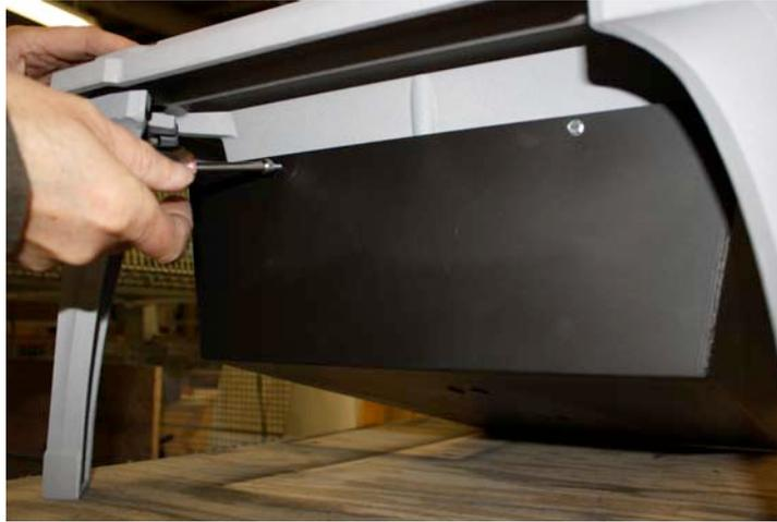
4. Install the front shield extension (the front extension has a double layer of sheet metal). Starting at the ash door end, line up the holes in the extension, the ash pan shield, and ash pan holder and start a sheet metal screw through all three pieces. Start sheet metal screws through each piece in the remaining two holes. The extension should angle up toward the front of the stove base.
