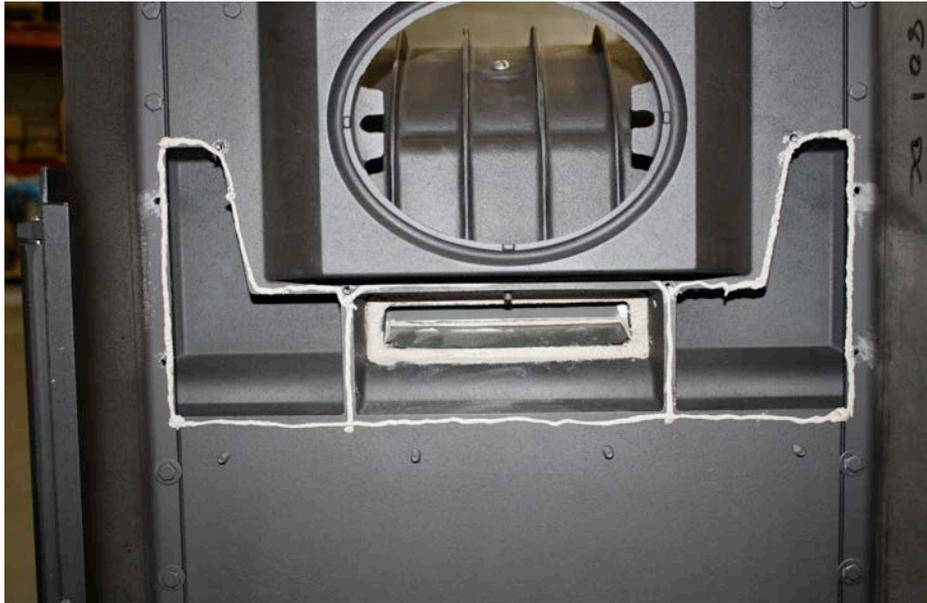
14. Use the four lower bolts as a guide to align the damper assembly with the back of the stove. Press the assembly into the cement evenly and gently pull up on the assembly to align all the holes. Start the two outside nuts at the bottom corners. Start the two bolts at the upper corners. Start the remainder of the nuts and bolts.
