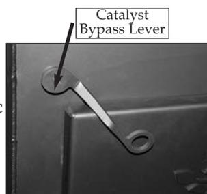
*The bypass lever interlocks with the door when the combustor is engaged (bypass closed). This safety feature makes it impossible to open the loading door without opening the bypass.*
