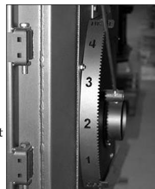
*The amount of combustion air available in the firebox is controlled by the damper lever.*
