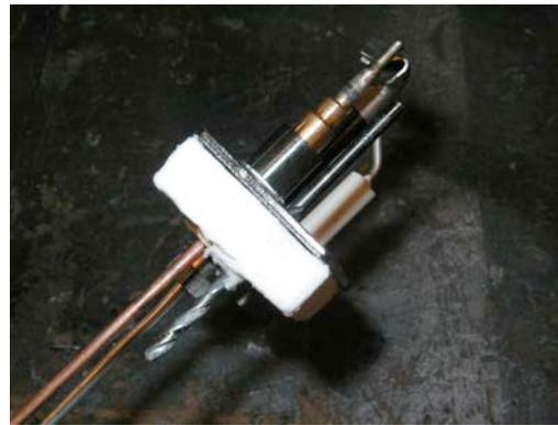
22. **Note: The open side of the pilot hood must face the burner pan to ensure proper stove operation.**
