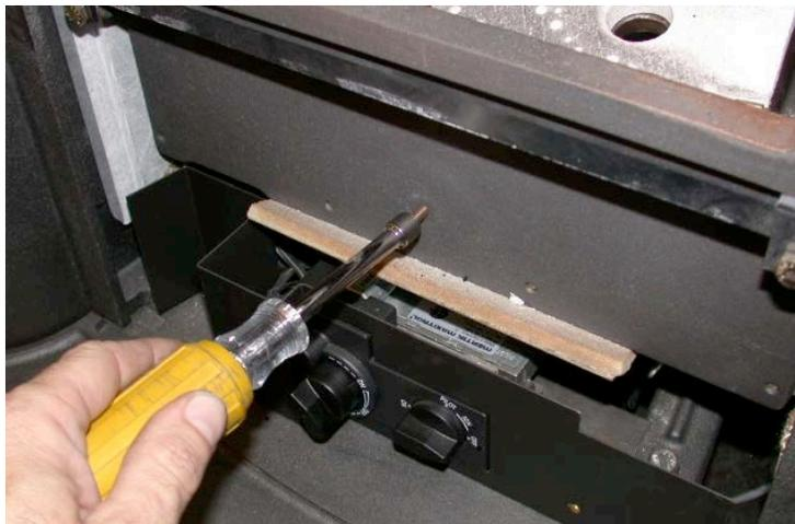
17. Lift the front edge of the burner pan and then pull the pan up and out of the firebox.
