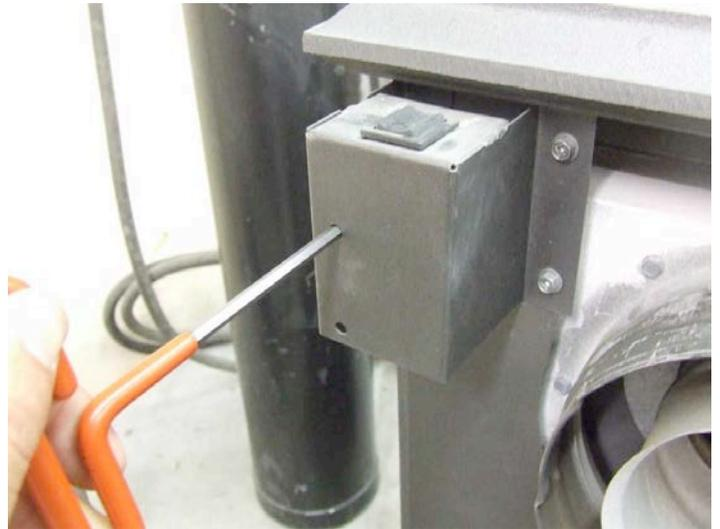
7. Remove the two screws to the right of the switch box with a 1/4" nut driver.
