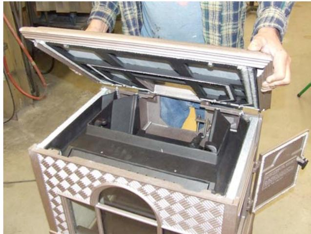
7. Use a  $\frac{1}{2}$ " socket to remove the two bolts that hold the front of the combustor pan to the front wall of the stove.
