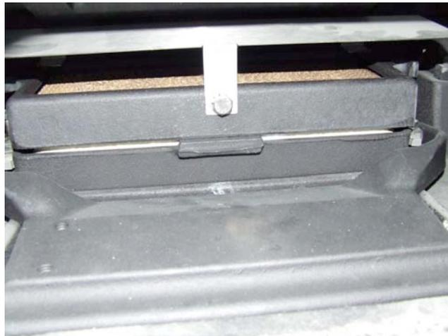
4. Remove the catalytic combustor. If you have not already removed the shipping bolts, use a 1/2" wrench to loosen them. They do not need to be re-installed.
