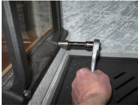
3. Install the new glass retainer with the same 1/2" socket (the pre-attached gasket provides a cushion where the retainer hits the soapstone piece). The bolts will either come pre-treated with anti-seize compound, or there will be a small packet of it in which to coat the threads. Tighten the bolts evenly and make sure they are secured properly.
